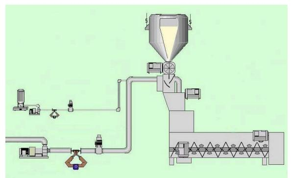
In mass flow metering the Master flow of product is sensed with a weigh belt, weigh feeder, impact scale, or centriflow meter. This type of measurement integrates the weight of the product with a tach signal from a conveyor or over a specified time period.
