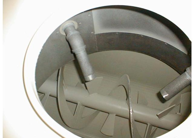
Spray into a screw conveyor: (fig 1)
