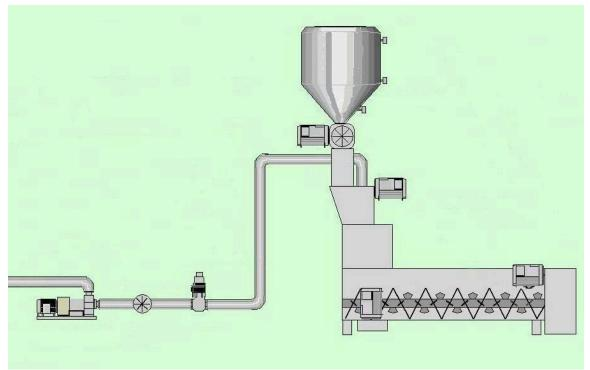
In volumetric metering the master flow of material is sensed by the number of revolutions of a screw conveyor, rotary feeder, or belt conveyor. We calibrate the material flow by measuring how much product has run through the system in a given amount of time. It is important to have a method to divert material from the process flow so that check weights can be done to confirm calibration.
