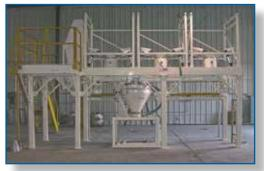
This system was designed for a company that produces industrial floor coverings. APEC provided the bulk bag dischargers, micro scale, tote staging system, bag dump station, and complete automation including motor control center and computer based recipe automation.
