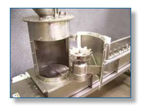
drum. This keeps the surrounding environment cleaner by preventing fugitive particles from escaping the machine. Another advantage of this machine is that it creates less back pressure than spray nozzles, so the pumps and other components last longer. This machine also works very well for food products such as nuts, cereal, and snacks.
